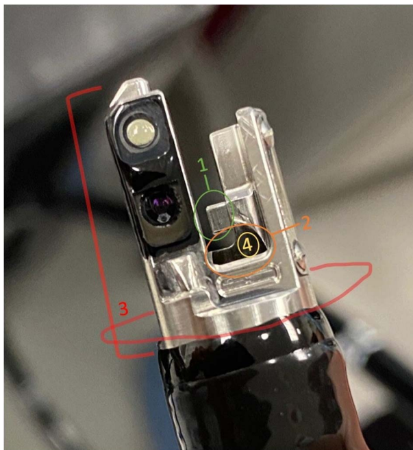
[1081] Figure 1. Sample locations: 1) The elevator tab, 2) instrument channel distal opening, 3) composite duodenoscope tip, and 4) the instrument channel. Samples 1-3 were collected with flocked swabs. The 4th was collected by flushing 25 mL of neutralizing buffer through the instrument channel, then scrubbing the channel with a brush, followed by another 25mL flush. The 50mL eluent was vacuum filtered through a 0.22-micron filter and plated on TSA. Duodenoscope serial numbers were recorded and one duodenoscope grew VRE in Phase 1 and Phase 2.
